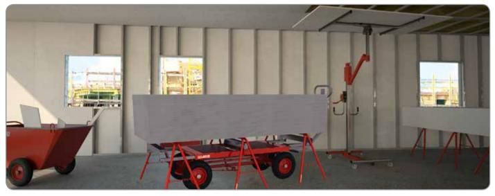
The Lift8 is a central part of our now classic system that handles the plasterboard from truck to assembly site without the need for a single person to handle a single sheet. Profitability is often described as a 50 % labour cost reduction with the added benefits that the plasterboard is off the floor preventing damage and poor ergonomics.
